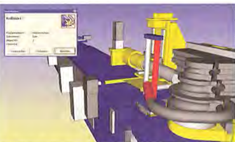
FIGURE 4 Simulated tube bending is not limited to single-head bending machines; simulation of multihead bending machines is also fairly common.
