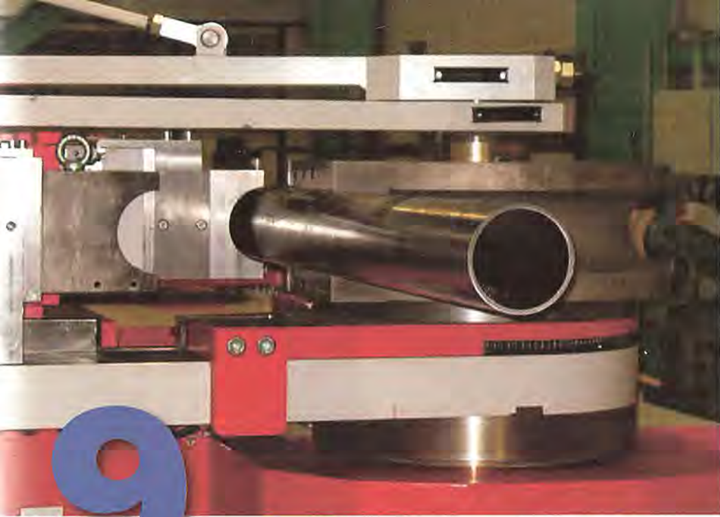
FIGURE 1 Tube bending simulation software ensures that a bending job can be done on a particular machine and that the bend is collision-free.
