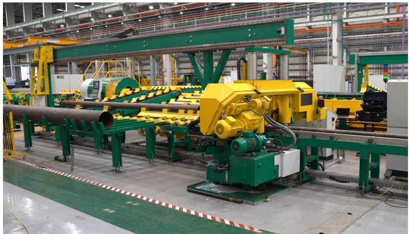
By automating the infeed and measuring, cycle times at a band-saw can be reduced significantly.
