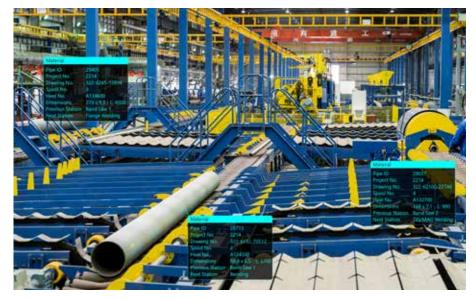
has a lot of high mix / low volume fabrication, meaning that there are a lot of different spool shapes, but each shape is fabricated only a few times, it is still possible to automate individual aspects of fabrication, such as cutting, edge preparation and the welding of fittings to straight pipes. This allows for significant time savings, greater accuracy, and lower risk of errors.
